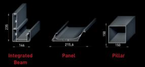
The Plus series is manufactured with four pillars up to a projection measure of 587,5 cm. Above this, one more pillar needs to be added for each of projection sides. The projection measure changes in multiples of 17,6 cm for both series.
